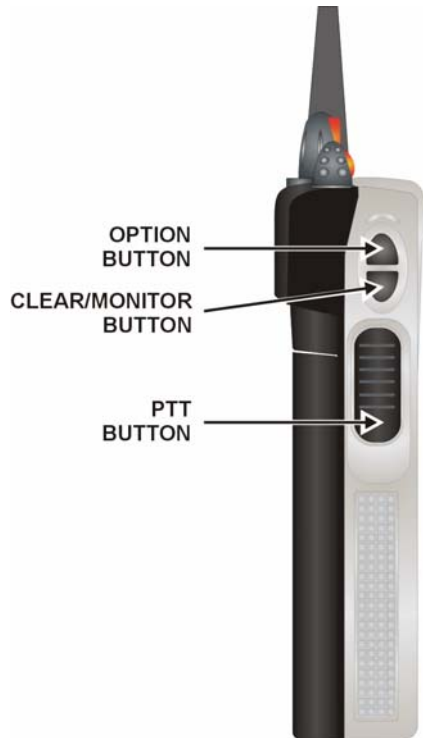
Figure 3 – Side View of Controls
